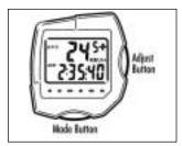
The Axiom is equipped with 2 buttons that control the function of the unit.
