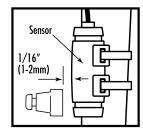
1. Position the axiom unit to the inside of either the right of left fork blade anywhere from 3-6 inches up from the fork blade tip. Attach the axiom to the fork blade with the quick ties but do not tighten the ties completely until final adjustment is complete.
